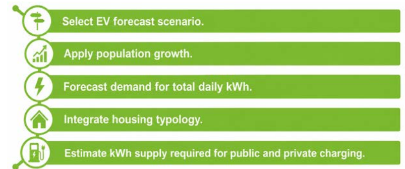
Figure 8 Steps in estimating future EV charging demand
