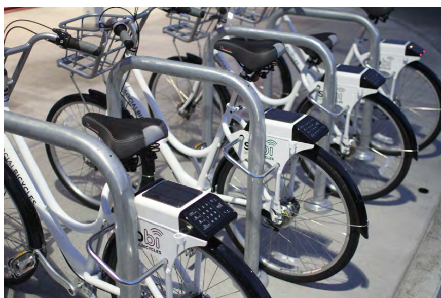
Figure 5 Solar panels are used to power on board technology
