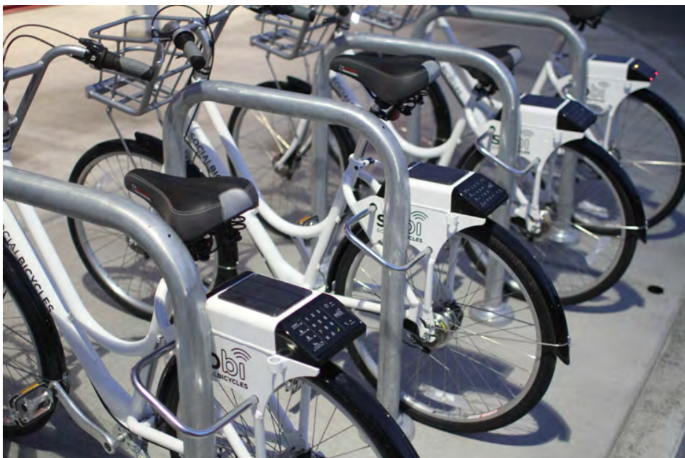
Figure 27 GPS enables operators to offer bicycles without docks
